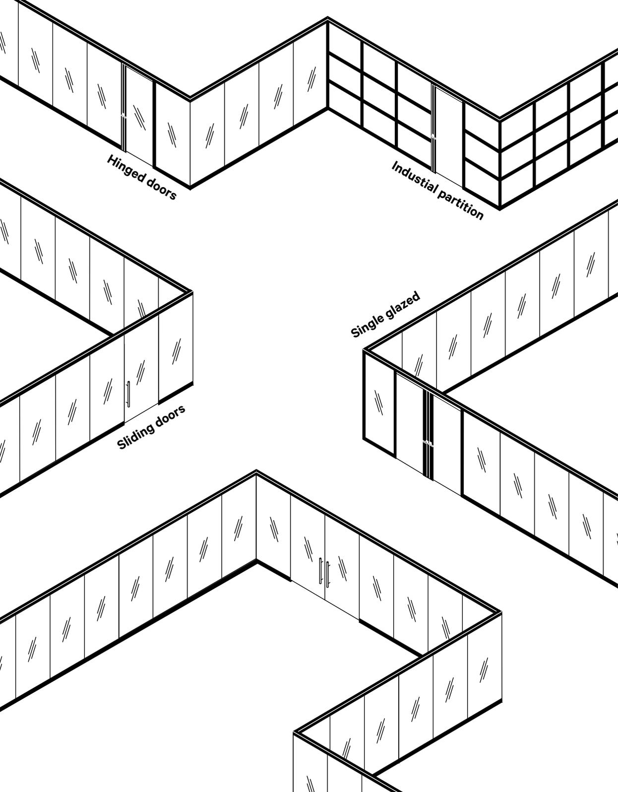
**WE is a single-glazed partition wall with a total thickness of 45 mm and 1 ¾ inches, available basic or industrial. In addition to the standard, many other glasses are available on request: extra-clear, acid-etched or screen-printed in various colors, with translucent colored PVB, LCD or with fabric interior.**
